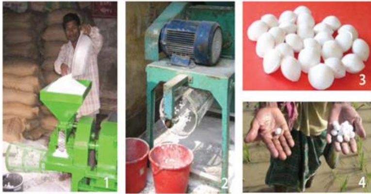
1) Prilled urea is poured into a briquetter. 2) A briquetter produces briquettes. 3) FDP briquettes. 4) The relative size of briquettes is shown.
